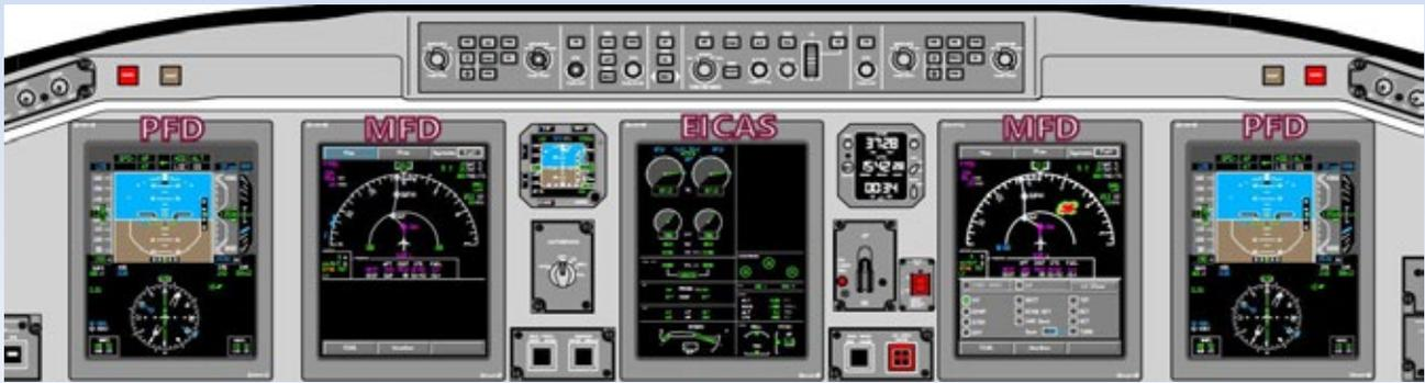
**Sistema EFIS (Electronic Flight Instrument System)**
